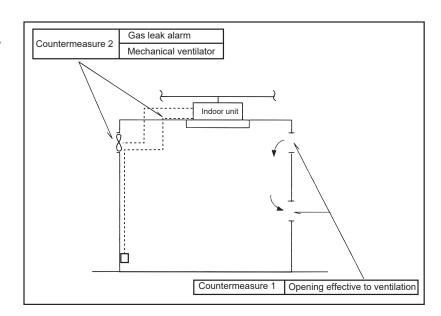
The installer and system specialist shall secure safety against leakage according to local regulations or standards. The following standards may be applicable if local regulations are not available.
