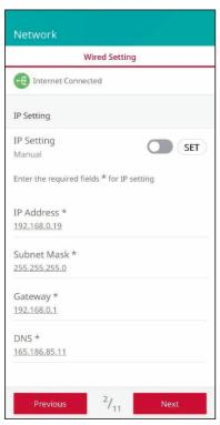
When the [Connection Type] option in the [Connection Status] is set to [Wired]. Wired connection options are displayed.
