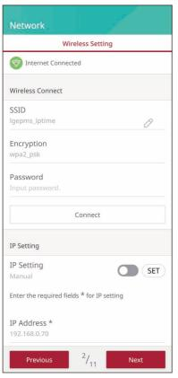
When the [Connection Type] option in the [Connection Status] is set to [Wireless]. Wireless connection options are displayed.
