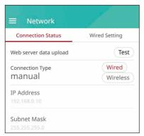
Select [Network] in [Installer Settings]. The current status of the network connection is displayed.
