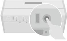
Push the WLAN button on bottom of ESS, and go to the menu Settings > WLAN and select ESS to connect. ESS WLAN password is 'WLAN Password' on right side of ESS device.
