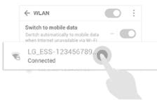
Push the WLAN button on bottom of ESS, and go to the menu Settings > WLAN and select ESS to connect. ESS WLAN password is 'WLAN Password' on right side of ESS device.
