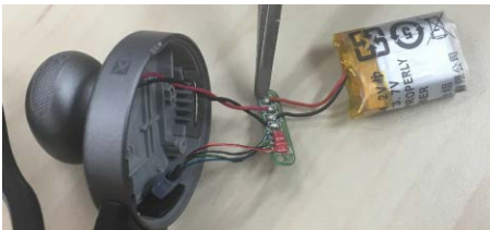
Remove battery wire.
