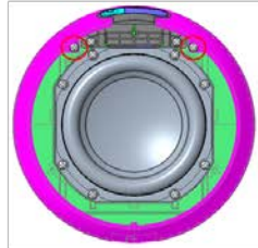
4) Disassemble of the Jersey Assy (2 screw)
