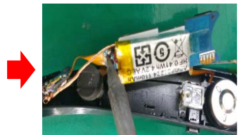
Remove battery wire.
