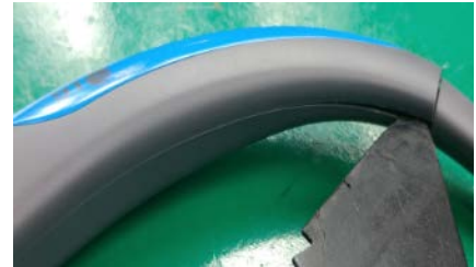
Insert the tool to the edge, and then disassemble from right to left.
