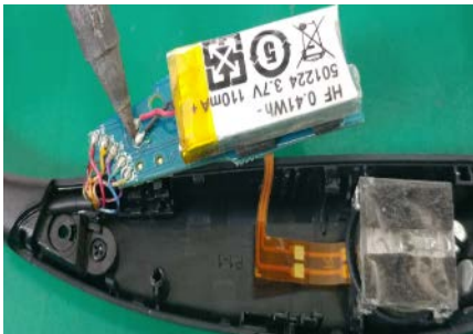
Remove battery wire.
