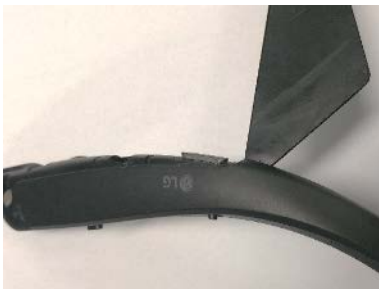
Insert the tool to the edge, and then disassemble from left to right .
