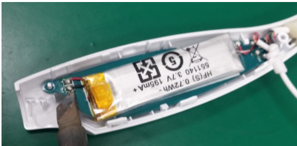
Remove battery wire.
