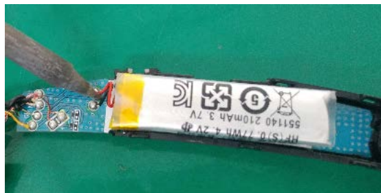
Remove battery wire.
