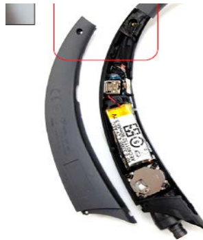
Insert the tool to the edge, and then disassemble from right to left.
