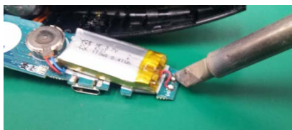
Remove battery wire.
