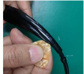
Insert the tool to the edge, and then disassemble right to left.
