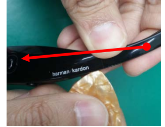
Insert the tool to the edge, and then disassemble from right to left..
