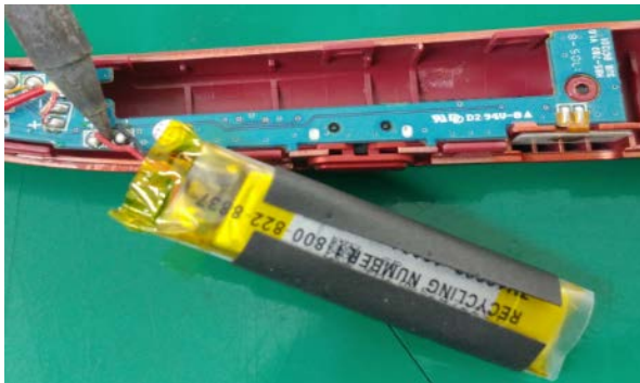
Remove battery wire.
