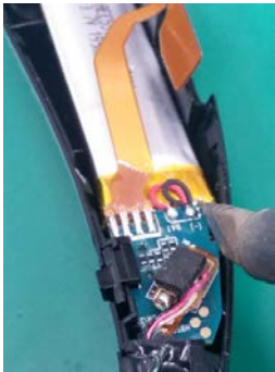
Remove battery wire.
