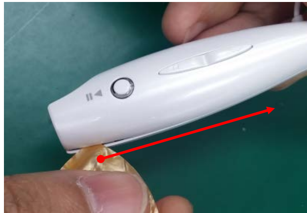
Insert the tool to the edge, and then disassemble from left to right.
