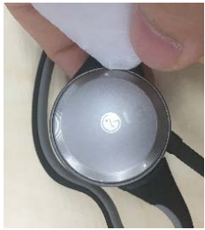
Using a tool, detach Upper case.
