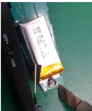
Remove battery wire.
