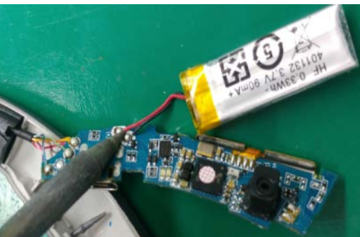
Remove battery wire.
