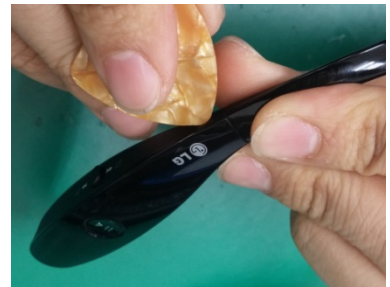
Insert the tool to the edge, and then disassemble from right to left..
