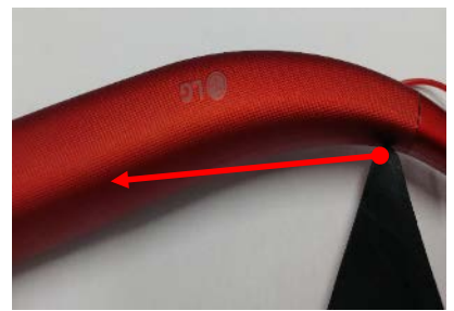
Insert the tool to the edge, and then disassemble from right to left.
