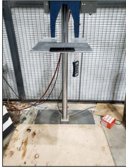
Photograph 18. Shock, Procedure IV – Transit Drop, Test Setup 1
