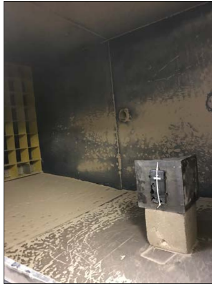
Photograph 13. Sand and Dust, Procedure I, Blowing Dust, Test Setup 5
