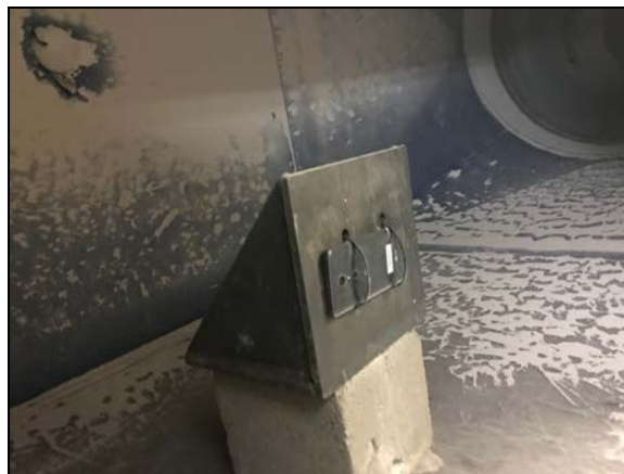
Photograph 11. Sand and Dust, Procedure I, Blowing Dust, Test Setup 3
