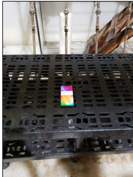
Photograph 7. Rain, Procedure III, Drip, Test Setup
