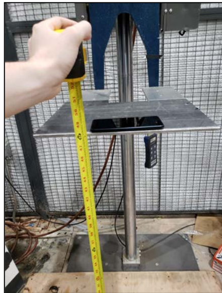
Photograph 19. Shock, Procedure IV – Transit Drop, Test Setup 2
