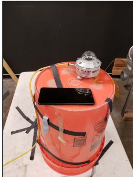
Photograph 6. Solar Radiation (Sunshine), Procedure I, Cycling, Test Setup
