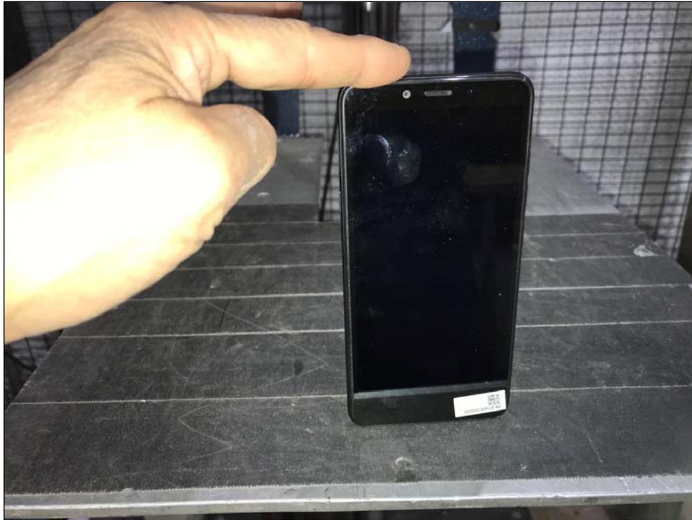
Figure 53: Method 516.6, Shock, Procedure IV - Transit Drop, Setup 6
