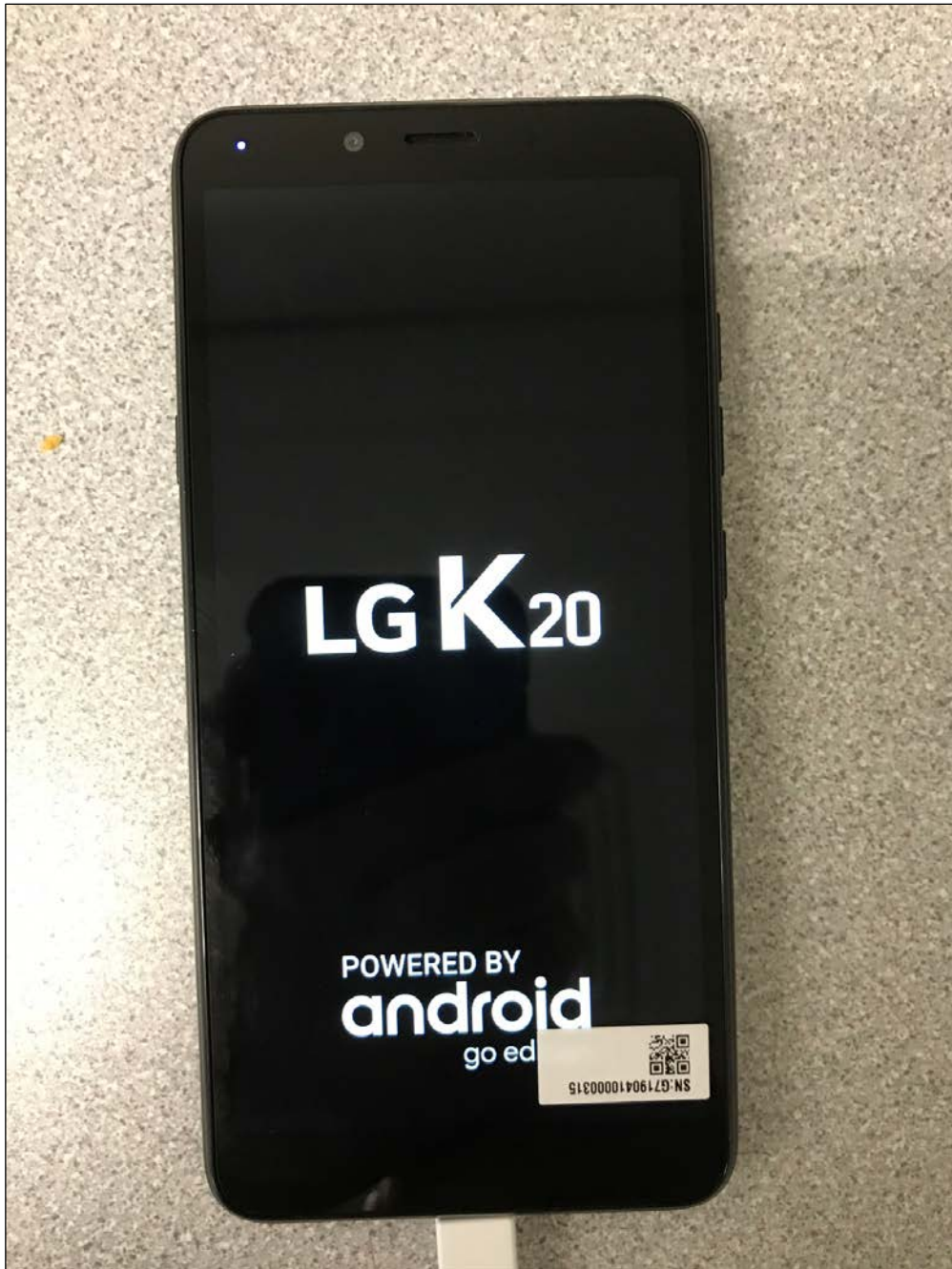
Figure 30: Method 507.5, Humidity, Procedure I, Post Test 1
