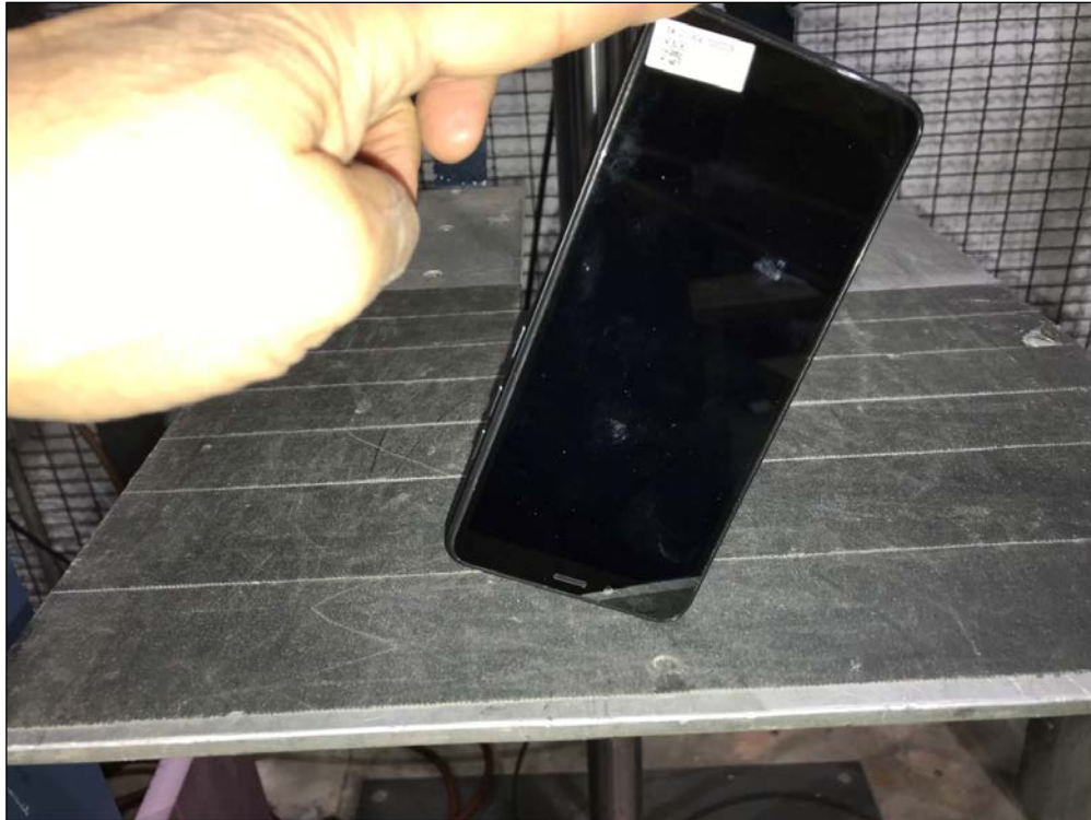
Figure 56: Method 516.6, Shock, Procedure IV - Transit Drop, Setup 9
