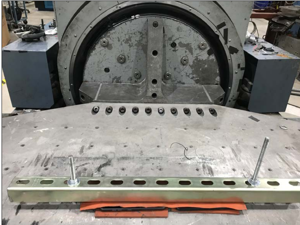
Figure 42: Method 514.6, Category 4 - Truck/Trailer/Tracked - Restrained Cargo, Setup Transverse
