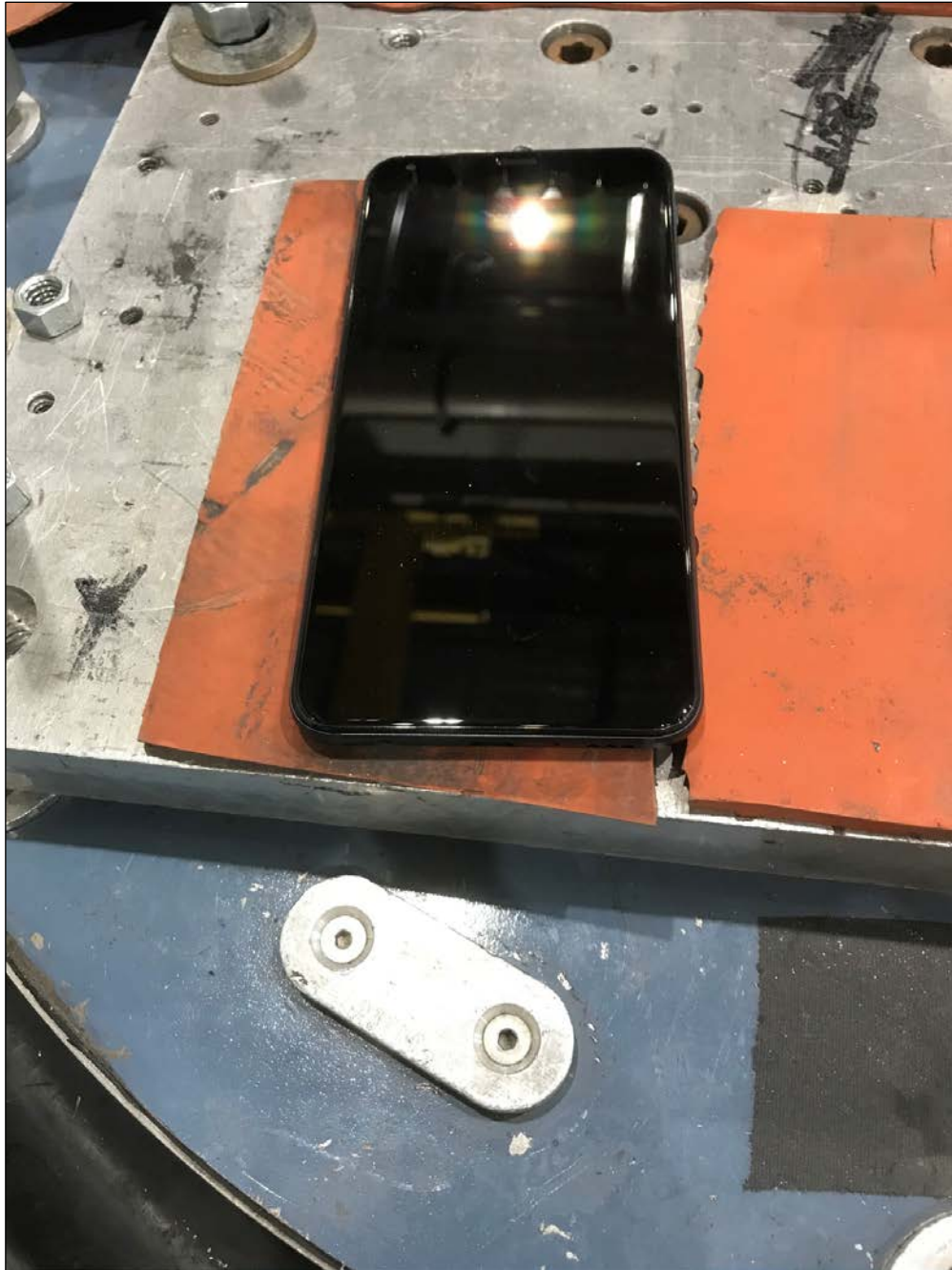
Figure 43: Method 514.6, Category 4 - Truck/Trailer/Tracked - Restrained Cargo, Setup Vertical
