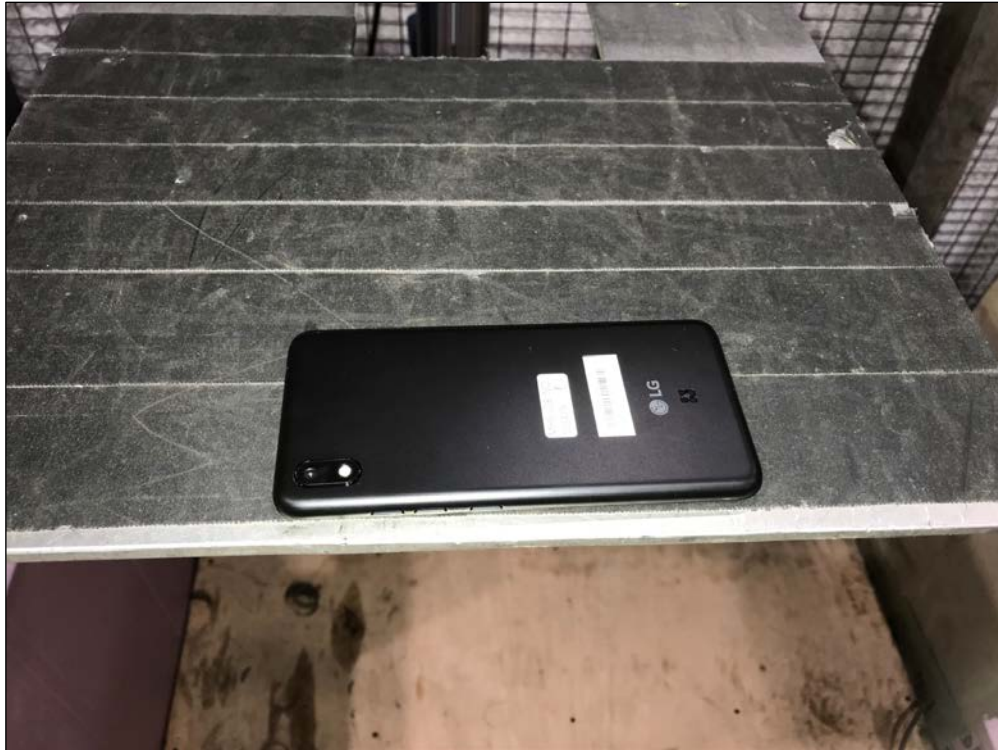
Figure 48: Method 516.6, Shock, Procedure IV - Transit Drop, Setup 1
