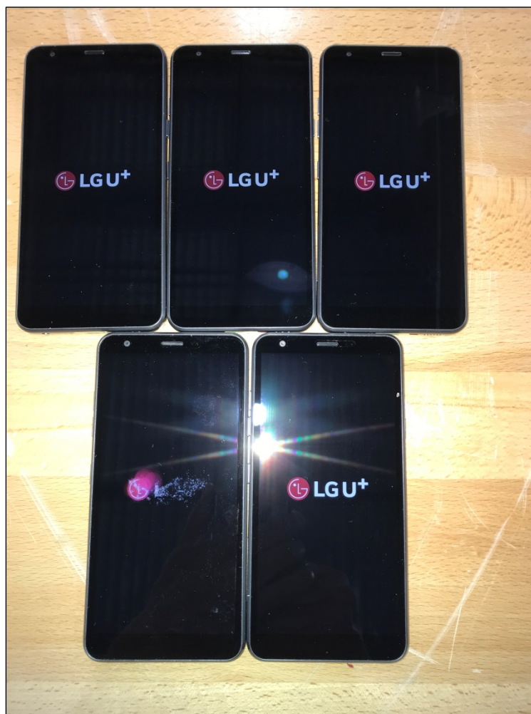
Figure 46: Method 516.6, Shock, Procedure IV - Transit Drop, Pretest 1
