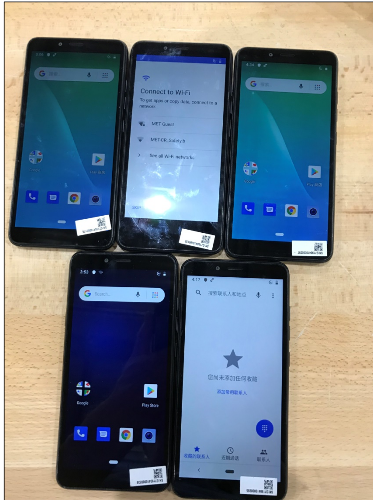
Figure 59: Method 516.6, Shock, Procedure IV - Transit Drop, Post Test 2
