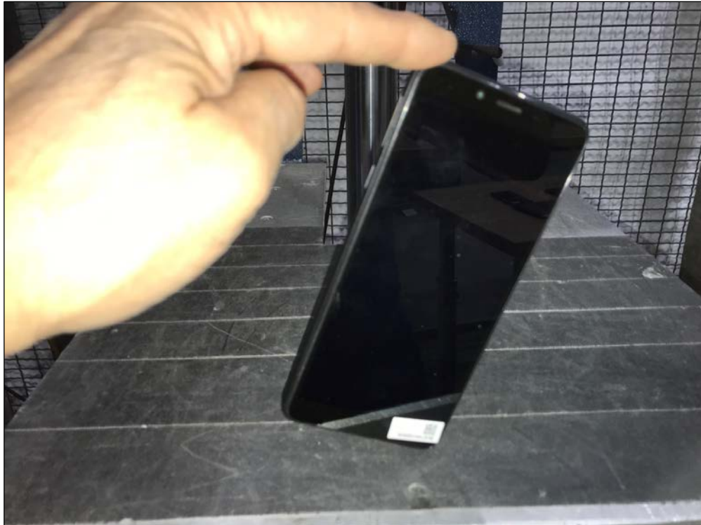
Figure 55: Method 516.6, Shock, Procedure IV - Transit Drop, Setup 8
