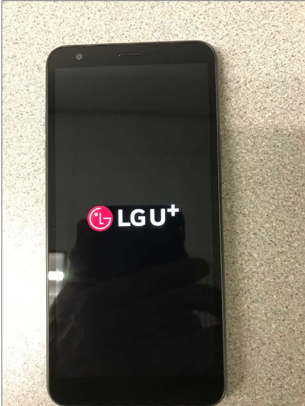
Figure 26: Method 503.5 - Temperature Shock, Procedure I-C – Multi-Cycle Shocks, Post Test
