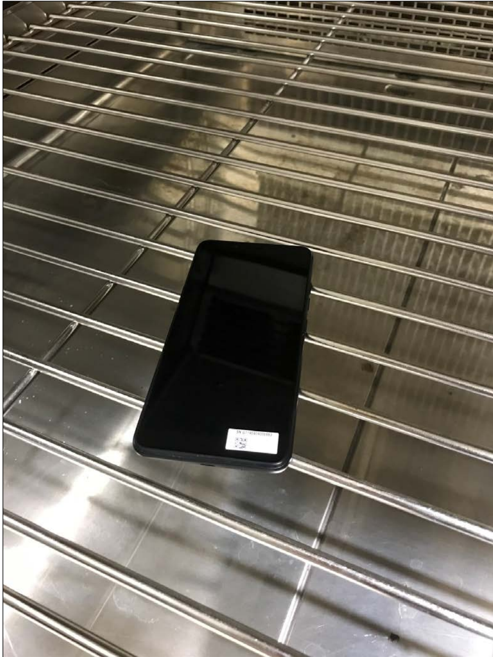
Figure 13: Method 502.5 - Low Temperature, Procedure I – Storage, Setup
