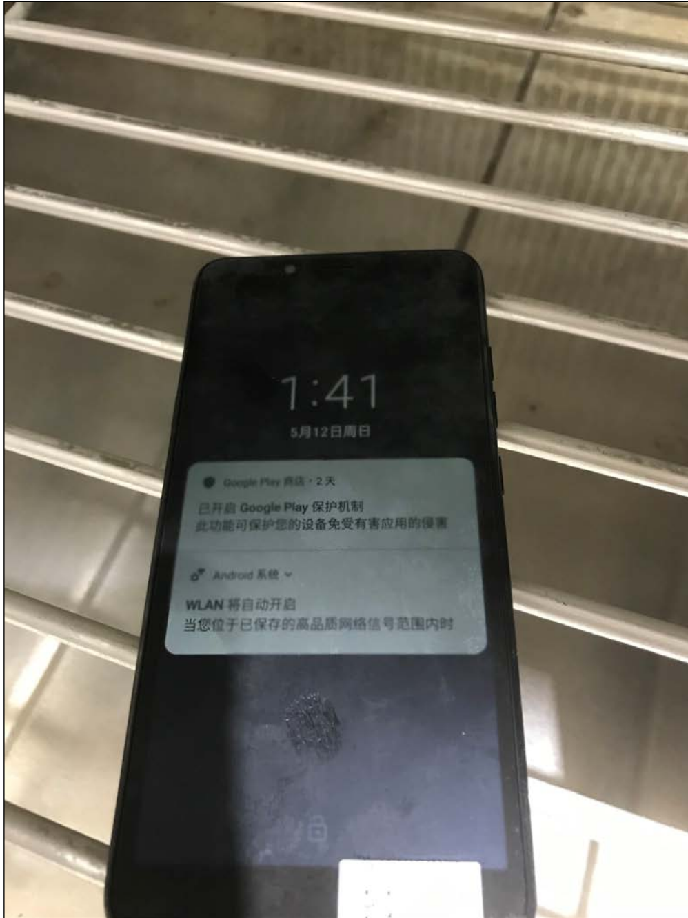
Figure 9: Method 501.5 - High Temperature, Procedure II – Operation, Setup
