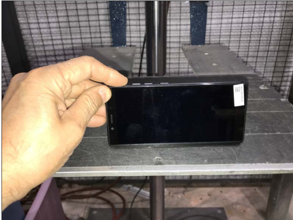
Figure 50: Method 516.6, Shock, Procedure IV - Transit Drop, Setup 3
