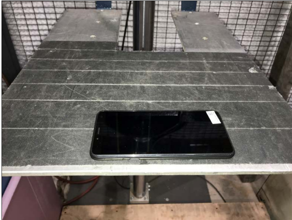
Figure 49: Method 516.6, Shock, Procedure IV - Transit Drop, Setup 2
