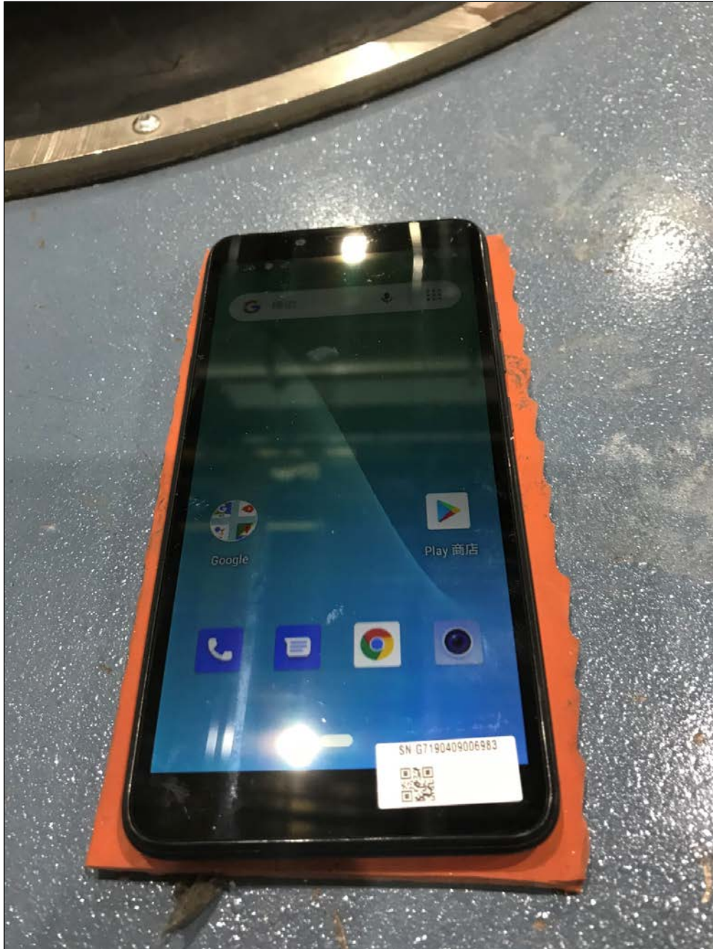
Figure 44: Method 514.6, Category 4 - Truck/Trailer/Tracked - Restrained Cargo, Post Test
