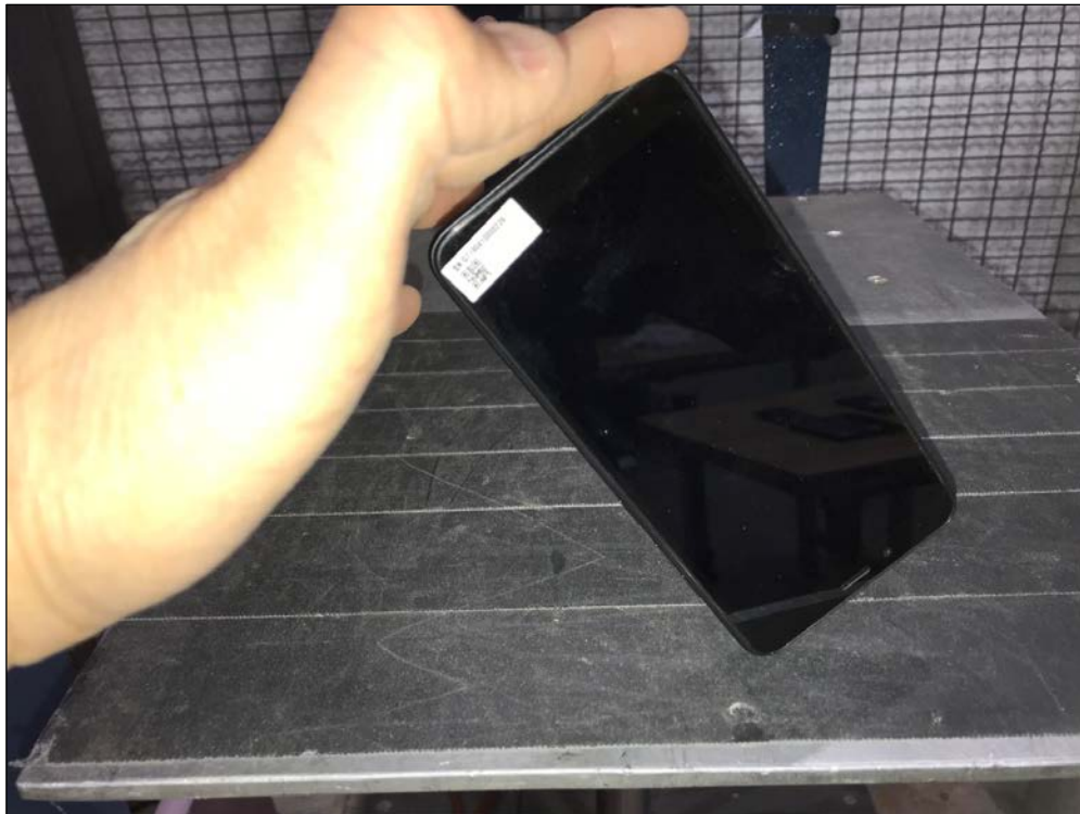
Figure 57: Method 516.6, Shock, Procedure IV - Transit Drop, Setup 10
