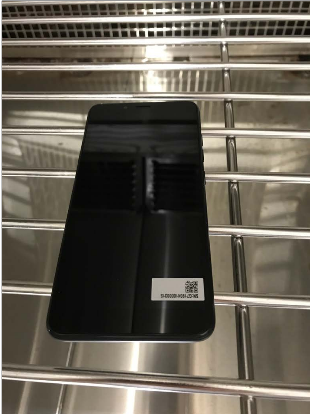
Figure 29: Method 507.5, Humidity, Procedure I, Setup in chamber
