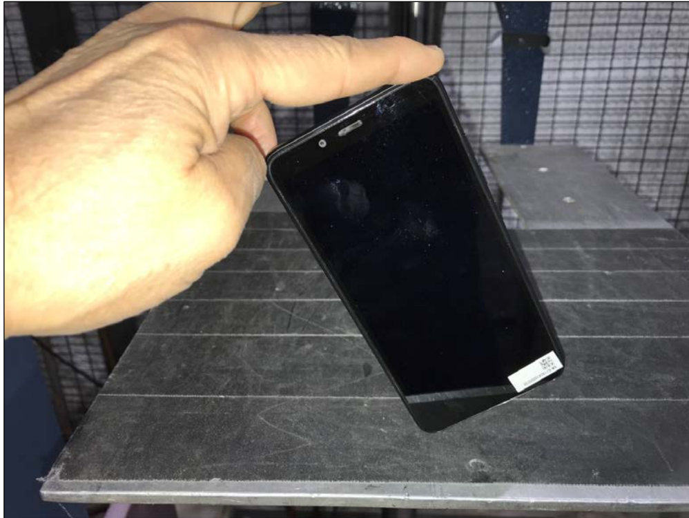
Figure 54: Method 516.6, Shock, Procedure IV - Transit Drop, Setup 7
