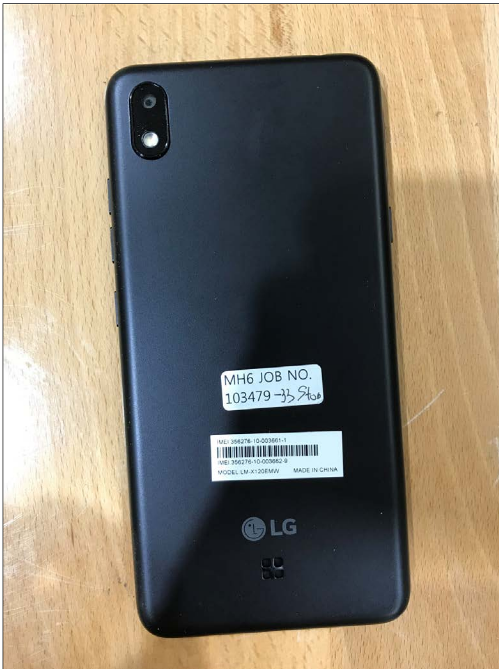
Figure 15: Method 502.5 - Low Temperature, Procedure I – Storage, Post Test 2
