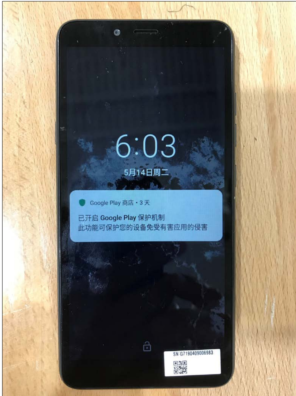
Figure 32: Method 507.5, Humidity, Procedure I, Post Test Verification
