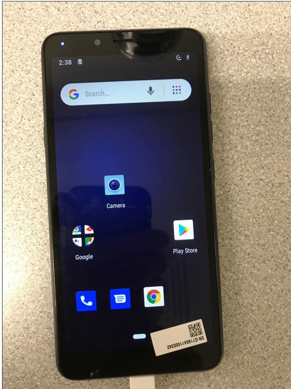
Figure 5: Method 501.5 - High Temperature, Procedure I – Storage, Post Test
