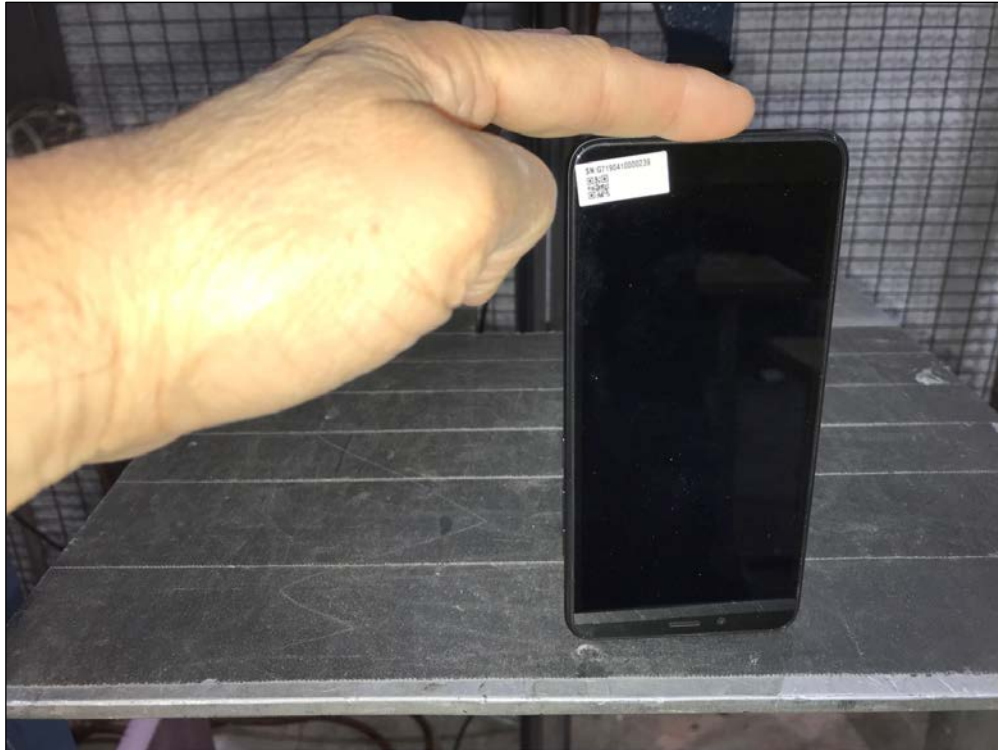
Figure 52: Method 516.6, Shock, Procedure IV - Transit Drop, Setup 5
