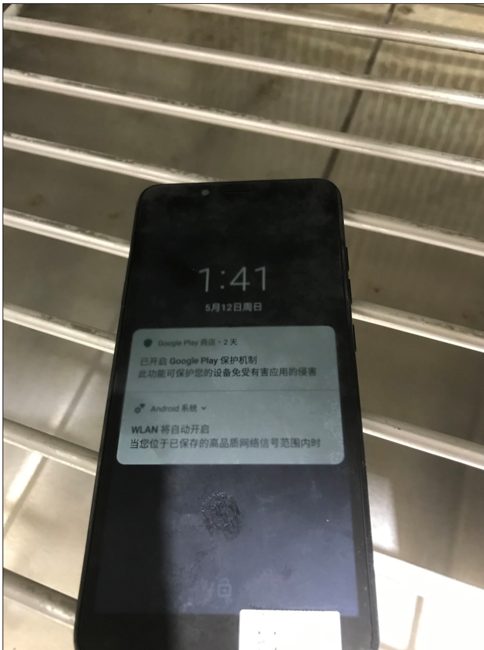
Figure 4: Method 501.5 - High Temperature, Procedure I – Storage, Setup in chamber
