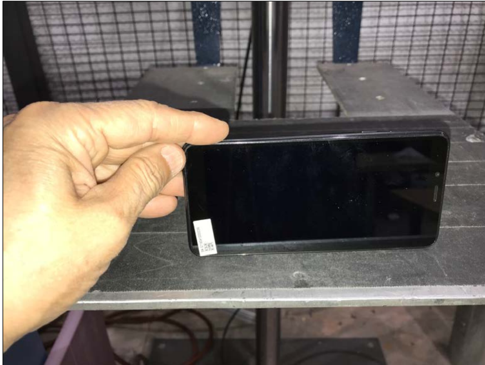
Figure 51: Method 516.6, Shock, Procedure IV - Transit Drop, Setup 4
