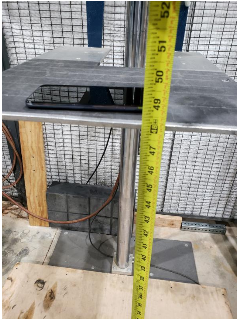
Figure 24: Method 516.6, Shock, Procedure IV - Transit Drop, Drop setup
