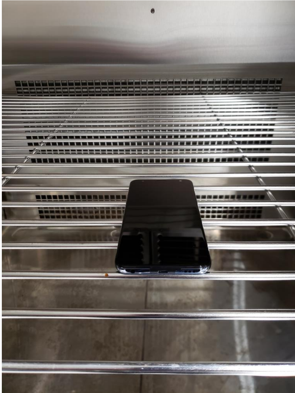
Figure 12: Method 507.5, Humidity, Procedure I, Natural Cycles, Storage Test Setup
