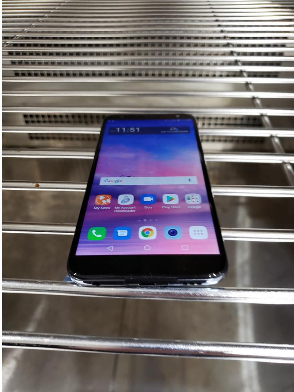
Figure 8: Method 503.5, Temperature Shock, Procedure I-C – Multi-Cycle Shocks, Test Setup
