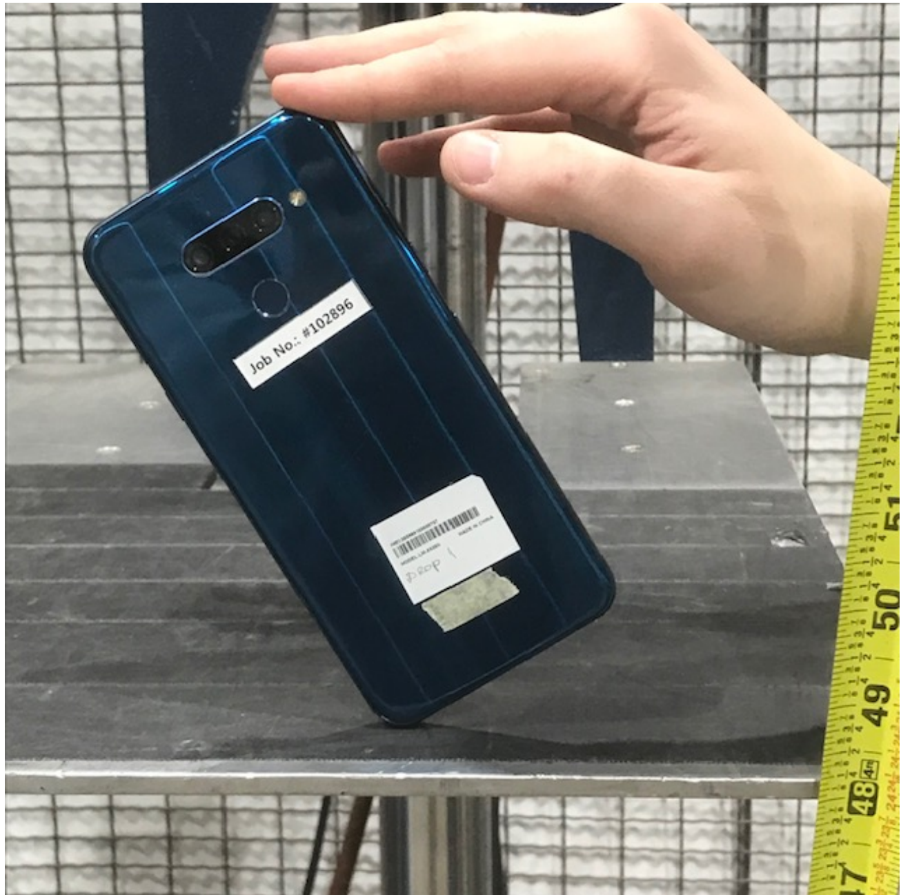
Figure 50: Shock, Procedure IV - Transit Drop, Setup 9
