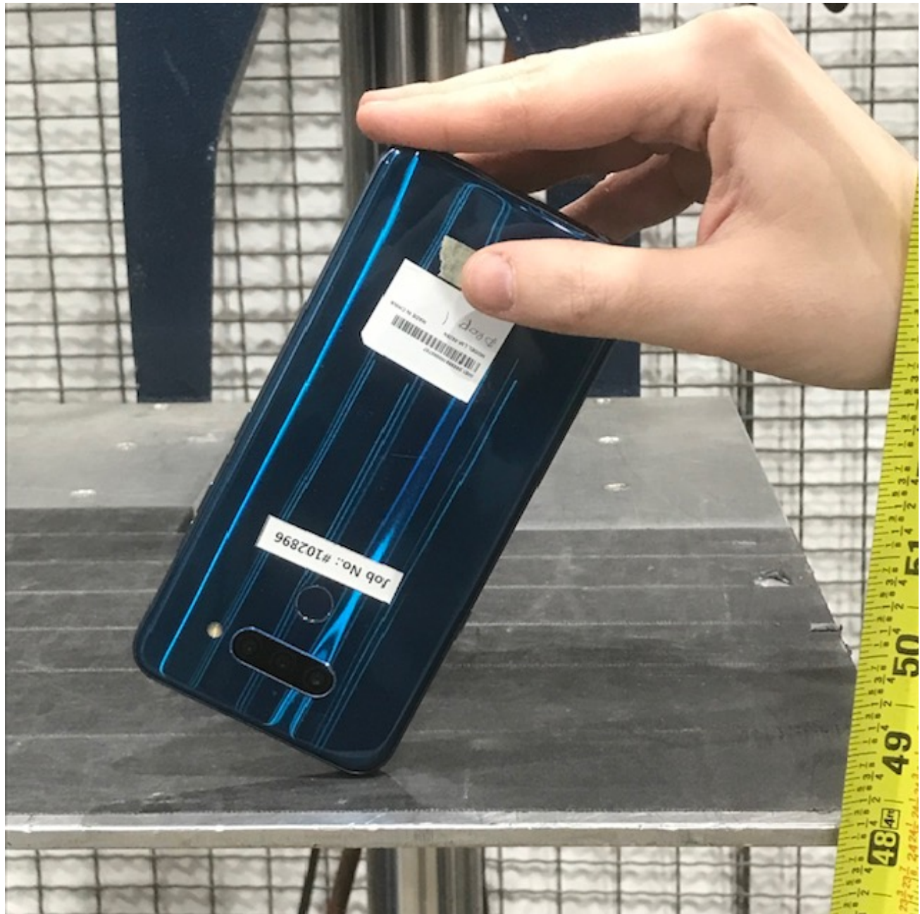
Figure 51: Shock, Procedure IV - Transit Drop, Setup 10
