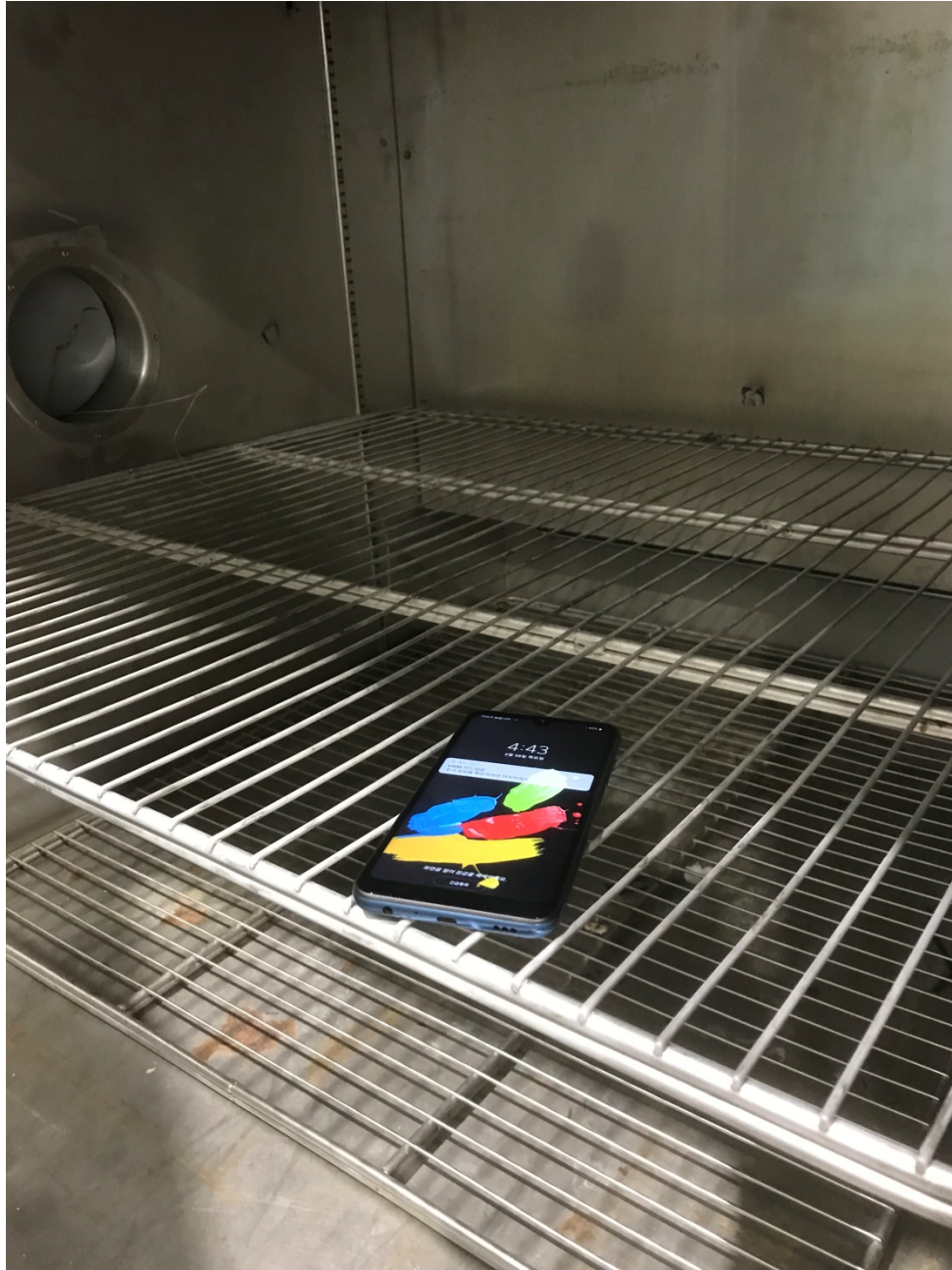
Figure 15: Temperature Shock, Procedure I-C, Setup In Chamber H3, 43°C
