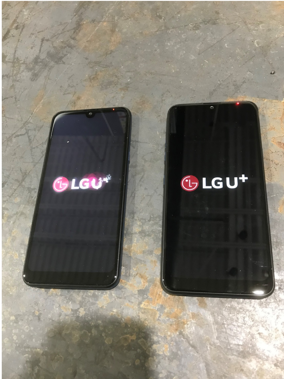
Figure 18: Temperature Shock, Procedure I-C, Post Test
