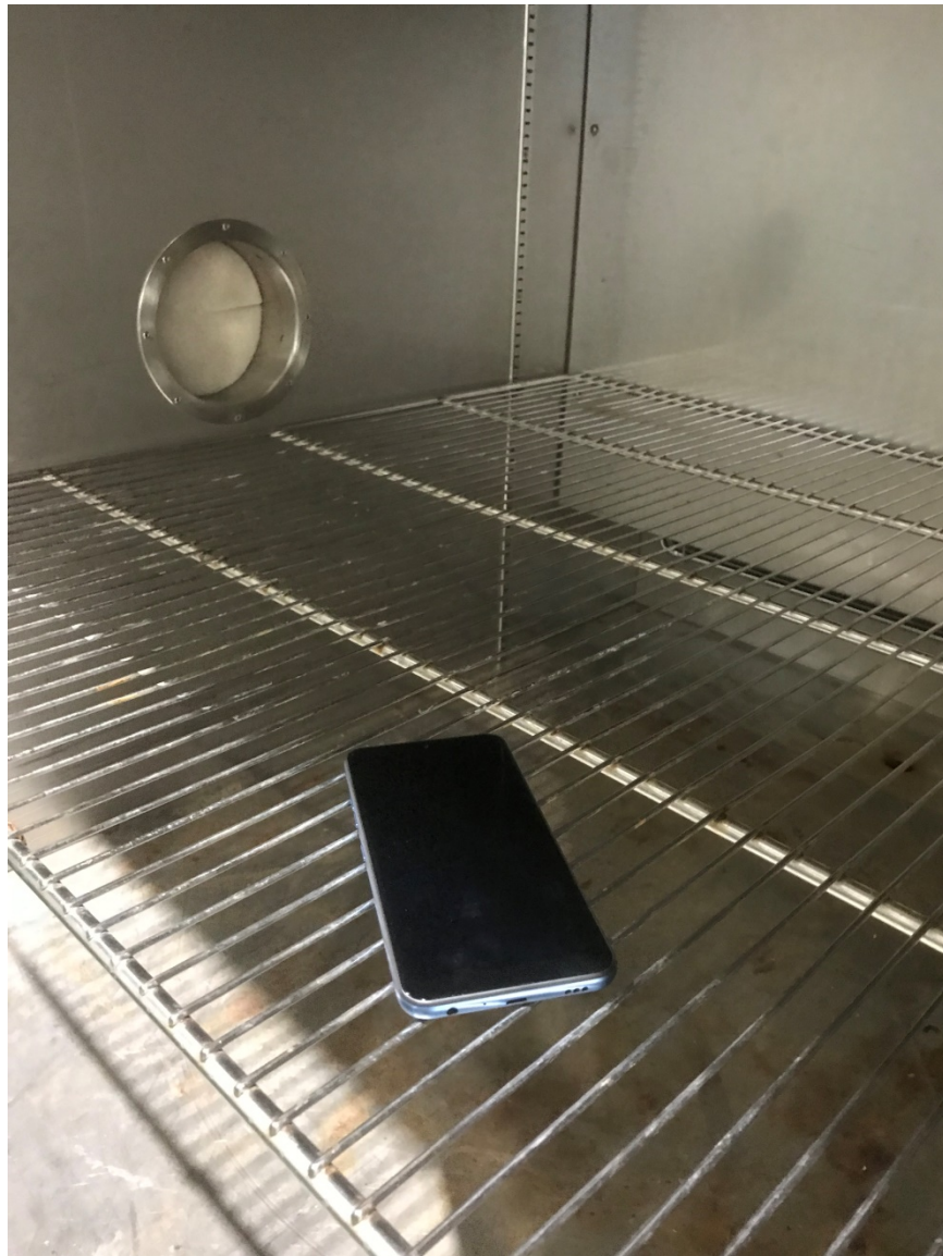
Figure 17: Temperature Shock, Procedure I-C, Setup In Chamber H4, -21°C
