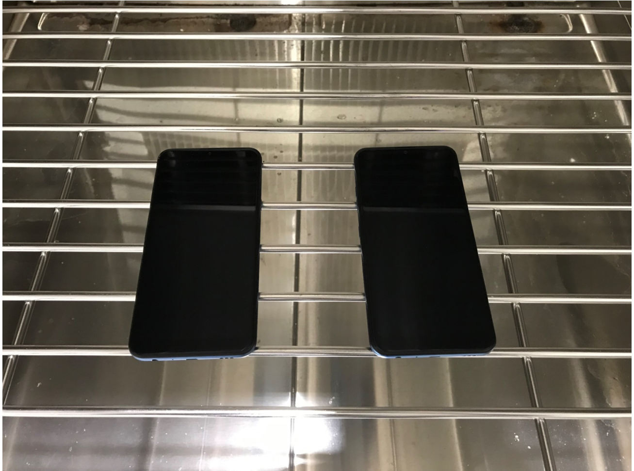
Figure 2: High Temperature, Procedure I – Storage, Setup
