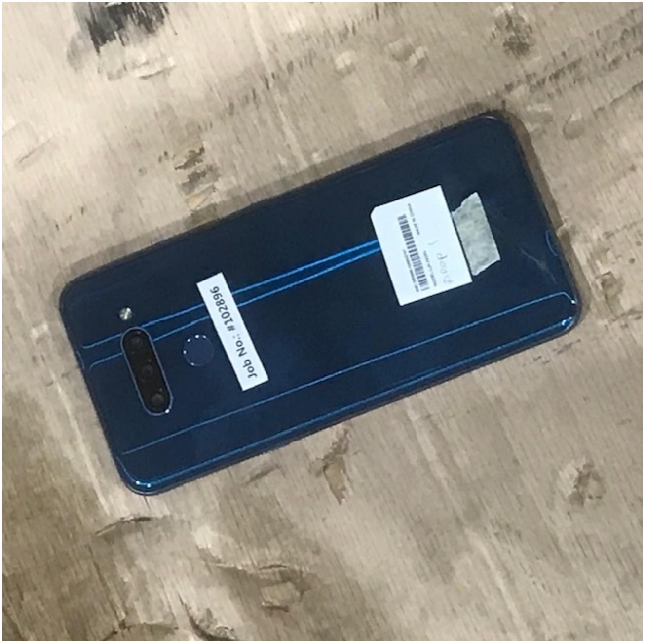
Figure 53: Shock, Procedure IV - Transit Drop, Drop On Plywood, 1
