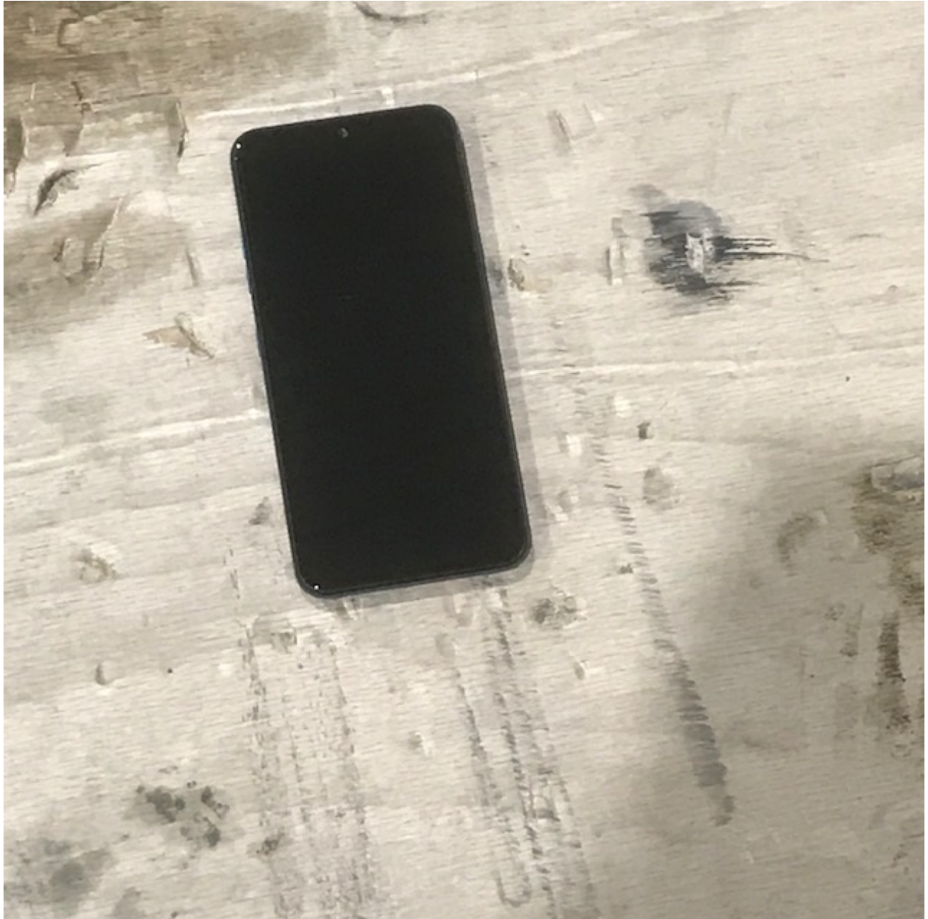
Figure 54: Shock, Procedure IV - Transit Drop, Drop On Plywood, 2
