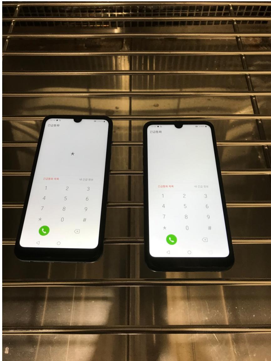
Figure 12: Low Temperature, Procedure II – Operation, Setup
