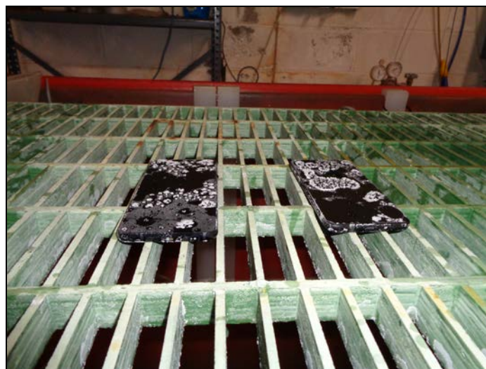
Photograph 11. Salt Fog, Test Setup (2)
