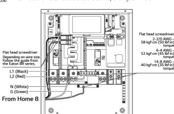
Insert the communication wires into the 6-position connectors.
