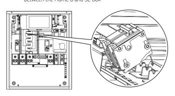
connect the AC conductors to the corresponding terminals
