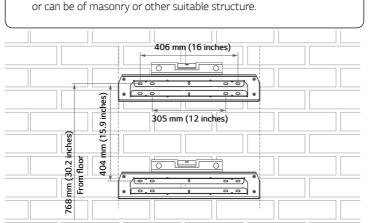
Affix the wall bracket to the wall with screws or anchors. Align the upper and lower brackets so that they are straight
