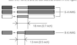
Connect the AC conductors to the corresponding terminals and connect the AC power ground
