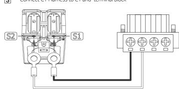
Plug the terminal block into the connector and tighten the screws
