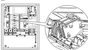
Pass the PV L1 cable from the PV inverter through the 200 A CT
