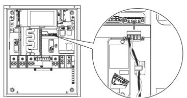
Arrange the power cables and fasten them using a cable tie.
