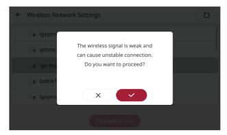
It is also necessary to check if the signal strength is sufficient under poor conditions (such as while the entrance or garage door is closed) during usage. If the signal is not strong enough to connect the internet, please consider installing the LG SE Box as close as possible to the router or install a WiFi range extender or Signal Booster.
